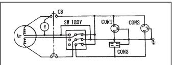
Figure 2. 120 V Simplified Diagram (Switch Up)
